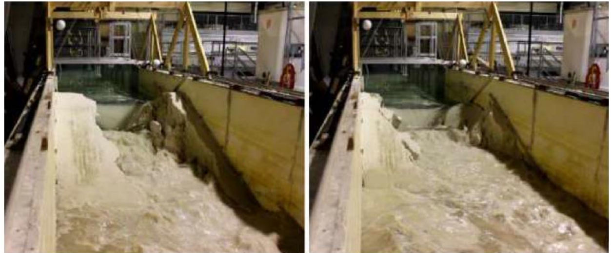
Fig. 12 Downstream oblique view of a typical dam during breach (Source: Walsh et al. 2019)
